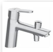
HANSAPRIMO one-hole single-lever mixer, DN 15 for rim-mounting 4951 2203 chrome connection with flexible hoses G 1/2, length 600 mm projection: 164 mm
